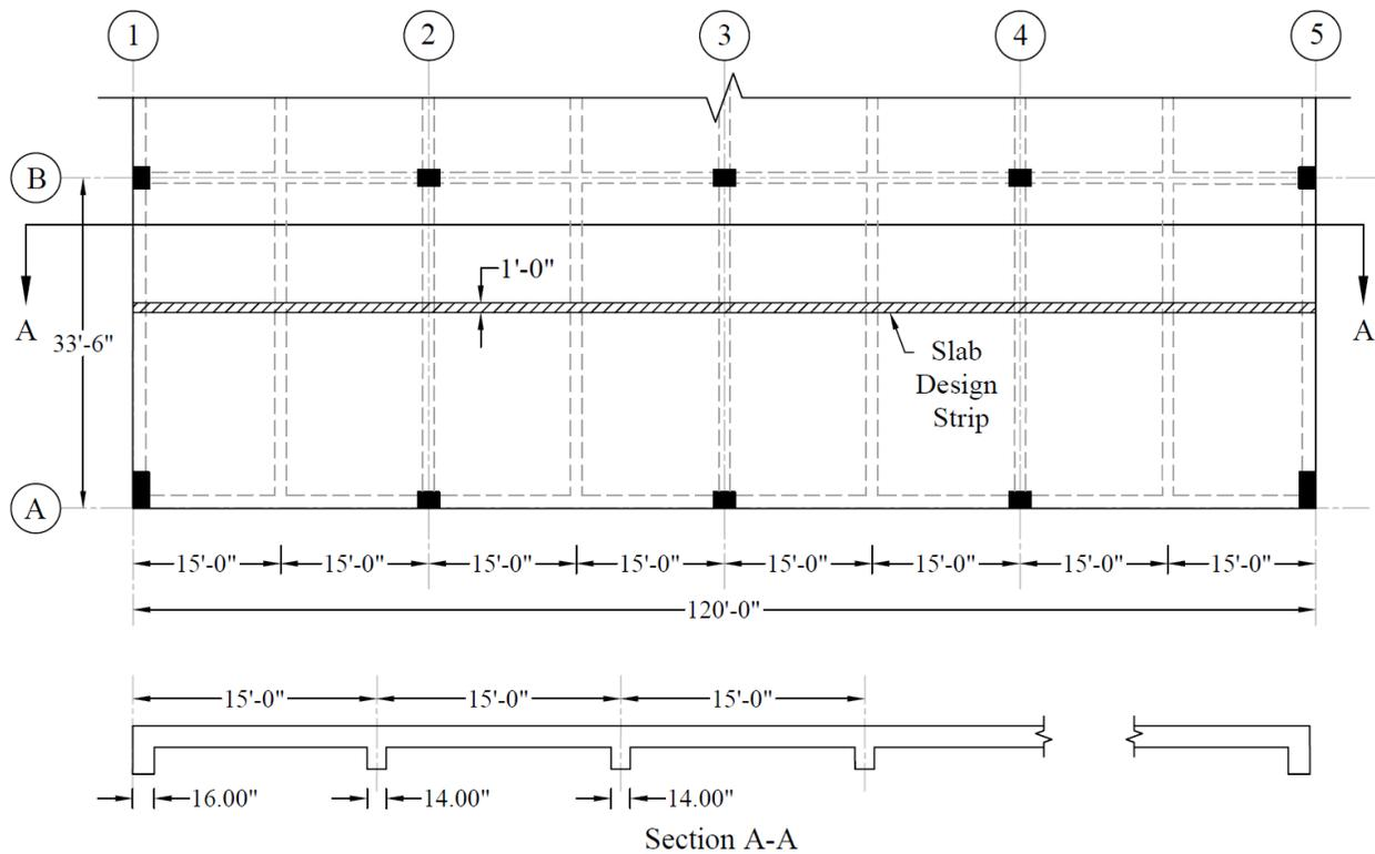
Figure 1 – Continuous One-Way Concrete Slab Floor System
