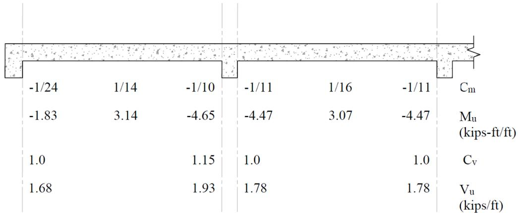
Figure 2 – Moment and Shear Coefficients and Design Values
