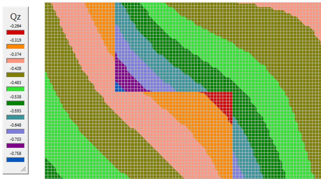
**Figure 3 - Service Load Combination S1 – Soil Bearing Pressure Contours (ksf) – v8.10**
