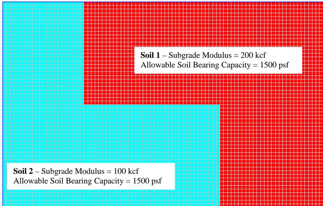
**Figure 1 – Plan View of Mat Foundation Slab with Dissimilar Soils**
