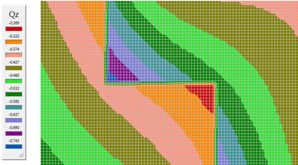
**Figure 4 - Service Load Combination S1 – Soil Bearing Pressure Contours (ksf) – v7.52 and prior**
