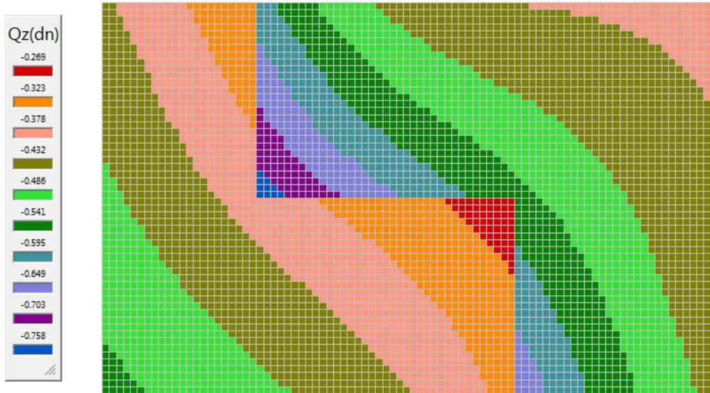
**Figure 2 – Envelope Pressure Down – Soil Bearing Pressure Contours (ksf) – v8.10 and prior**
