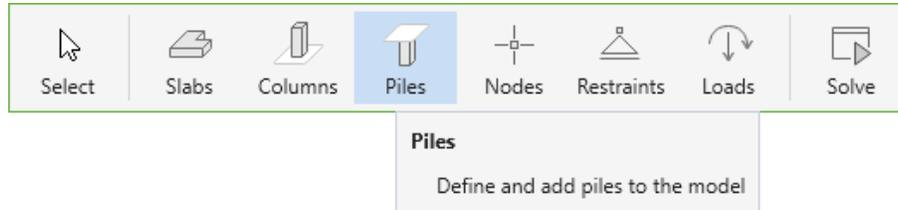
If you have already defined a **Pile** type in the DEFINITIONS dialog, simply select it from the LABEL drop down menu in the **Left Panel** to assign it to the model. You can also simply select the section type, enter the dimensions, select the required properties and start assigning, the corresponding pile definition created will automatically be added to the DEFINITIONS dialog.
