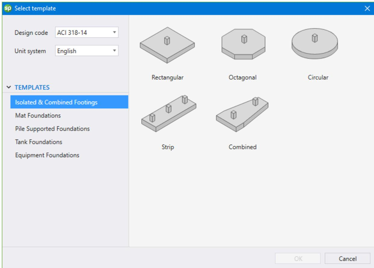
Here you can select the desired template along with the DESIGN CODE and UNIT SYSTEM. Double clicking on a template image or selecting a template image and clicking OK will open the **Template Module** and load the selected Template.
