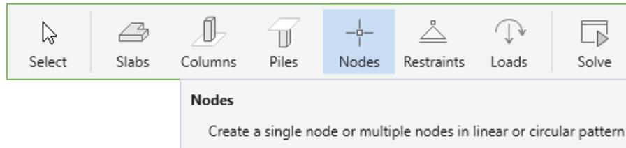
You can draw a **Single** node, nodes in **Linear** arrangement or nodes in **Circular** arrangement by using one of the following three tools in the **Nodes Left Panel**.
