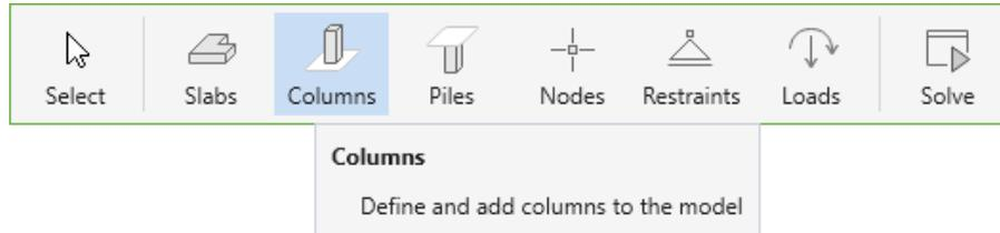
If you have already defined a **Column** type in the DEFINITIONS dialog, simply select it from the LABEL drop down menu in the **Left Panel** to assign it to the model. You can also simply select the section type, enter the dimensions and start assigning, the corresponding column definition created will automatically be added to the DEFINITIONS dialog.
