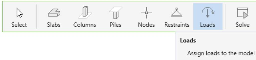
You can assign **Point** loads or **Area** loads by using one of the two options that are presented in the **Loads Left Panel**.
