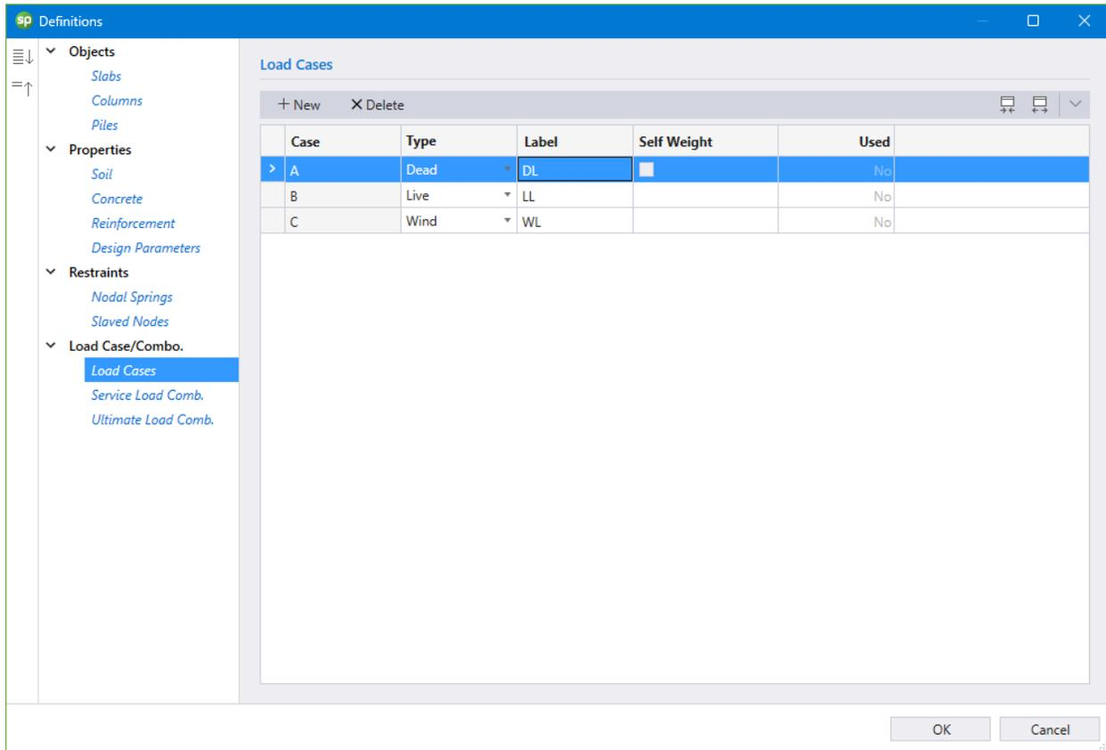
12. Click on **Service Load Combinations** from **Load Case/Combo.** to display the **Service Load Combinations** dialog box.
