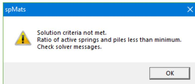
No results and contour views will be generated. The Program will retain the **Solver Messages Dialog** which will display a “Solution error: ratio of active springs and piles less than minimum = \_\_\_%” message for the first load combination that did not meet the criteria.
