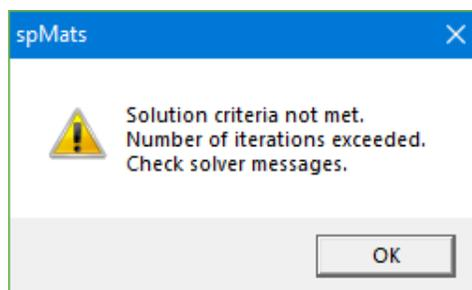
No output results and contour views will be generated. The Program will retain the **Solver Messages Dialog** which will display a “Solution error: Number of iterations exceeded” message for the first load combination that did not meet the criteria.
