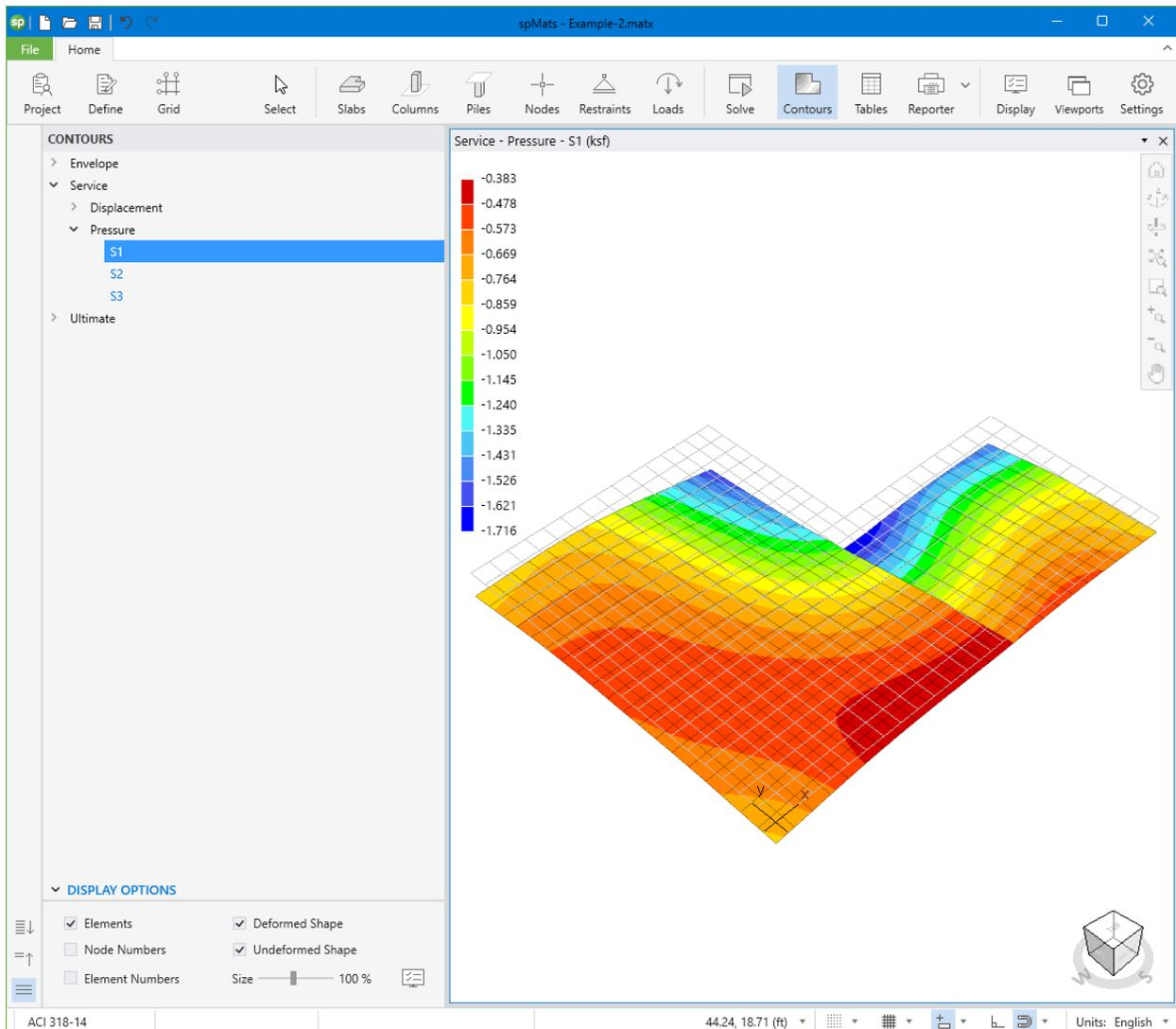
Soil pressure values in the contour view above differ along dissimilar soil boundaries. More information about Winkler's Foundation can be found in [Section 2.3.2.1](#).
