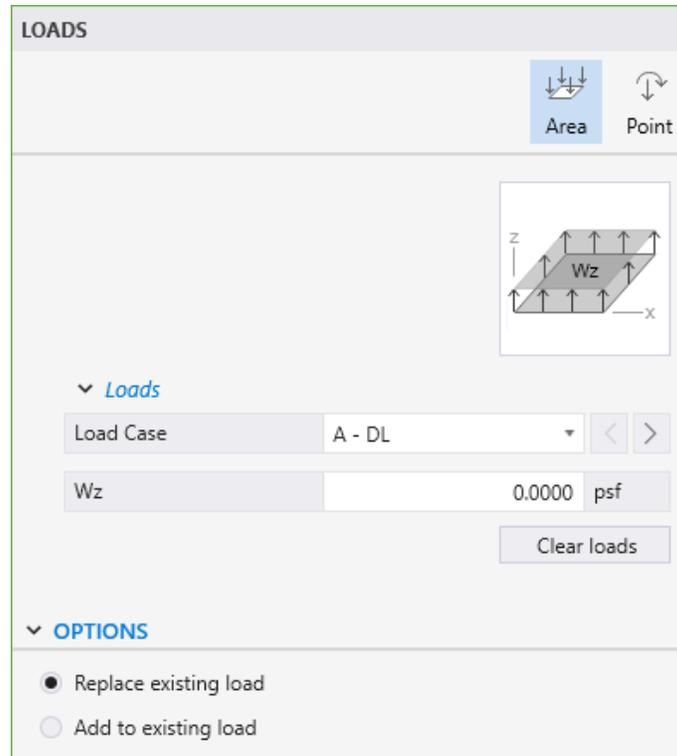
To assign an **Area** load, make sure that the **Area** command in the **Left Panel** is selected. The **Left Panel** should be displaying various **Area Loads** options.
