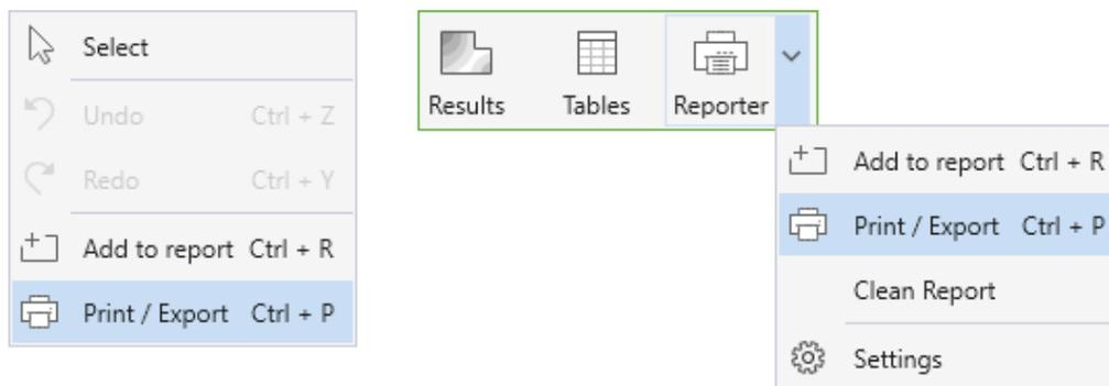
Alternatively pressing the “CTRL + P” also opens the **Print/Export Module**. Once the module is open the rest of the program is locked until the **Print/Export Module** is closed.
