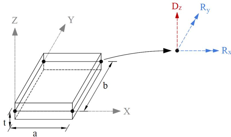
Figure 2.4 – Plate Finite Element
