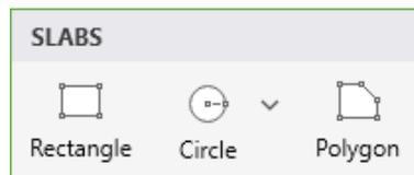
If you have already defined a slab type in the DEFINITIONS dialog, select it from the LABEL drop down menu in the **Left Panel** before you start drawing. You can also simply select the SECTION and PROPERTIES and start drawing, the corresponding definition created will automatically be added to the DEFINITIONS dialog.
