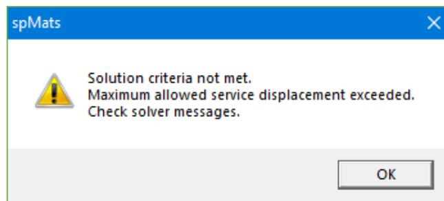
No output results and contour views will be generated. The Program will retain the **Solver Messages Dialog** which will display a “Solution error: Exceeded maximum allowed service displacement” message for the first service load combination that did not meet the criteria.
