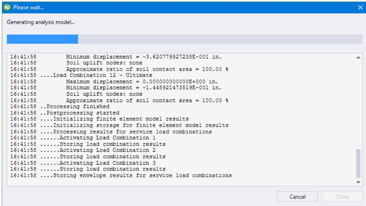
When the solution is successfully completed, a contour map showing downward displacement envelope is displayed. If the solution procedure fails, a message box appears. Detailed information on the solution can be found in the **Solver Messages Dialog** under **Tables Window**.
