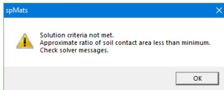
No output results and contour views will be generated. The Program will retain the **Solver Messages Dialog** which will display a “Solution error: Ratio of soil contact area is less than minimum = \_\_\_%” message for the first load combination that did not meet the criteria.
