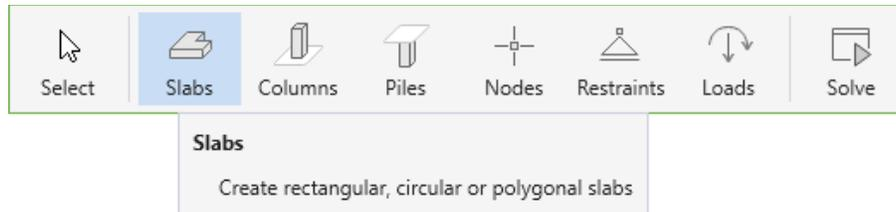
You can draw **Rectangular**, **Circular** or **Polygonal** slabs by using one of the following three tools in the **Slabs Left Panel**.
