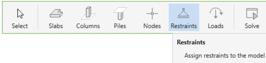
spMats considers restraints as nodal properties. It is possible to assign more than one kind of restraint to a node at the same time.
