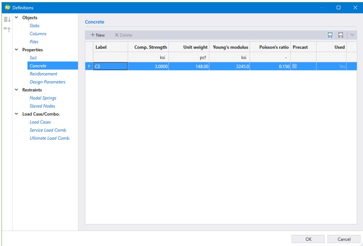
8. Click on **Design Parameters** from **Properties** to display the **Design Parameters** dialog box.
