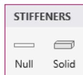
**Null** stiffeners are stiffeners without any properties. They only act as place holders for linear loads and supports, and do not contribute to the model structurally.
