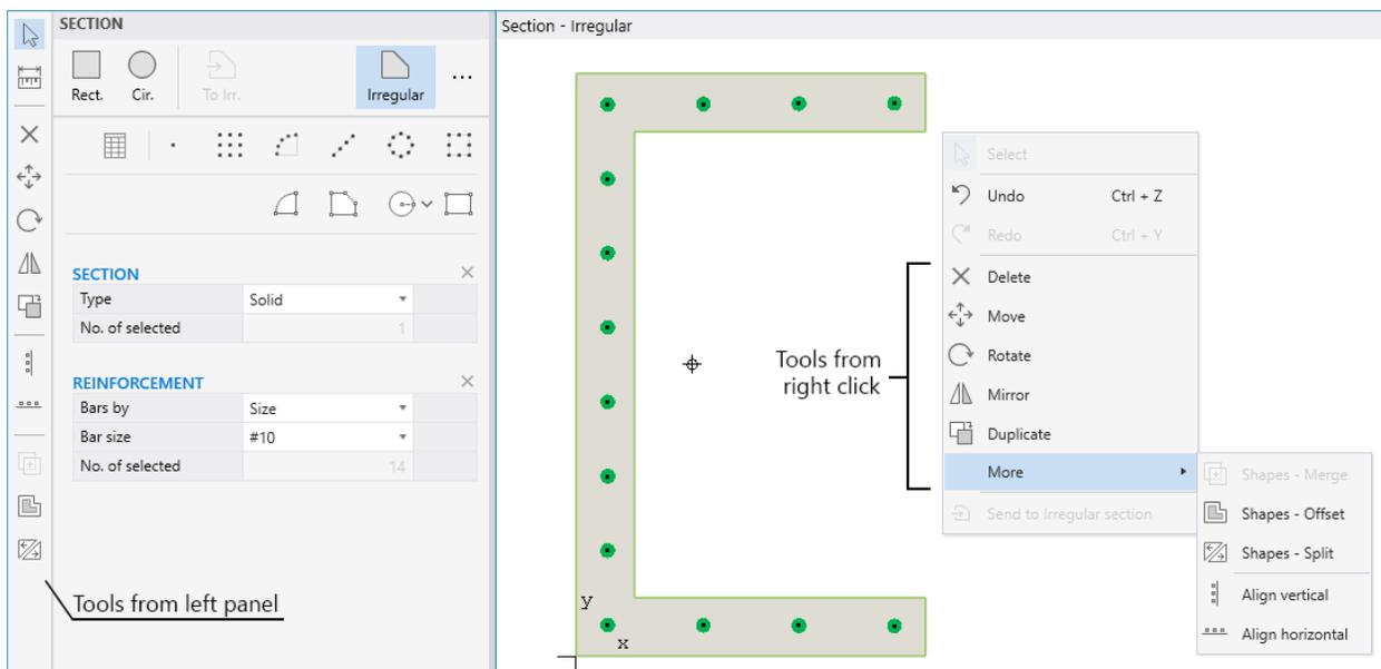
A convenient method for modeling and editing complex sections is to draw base shapes that overlap to create the desired final shape. The MERGE tool can be used to combine the component shapes and avoid any geometric errors.
