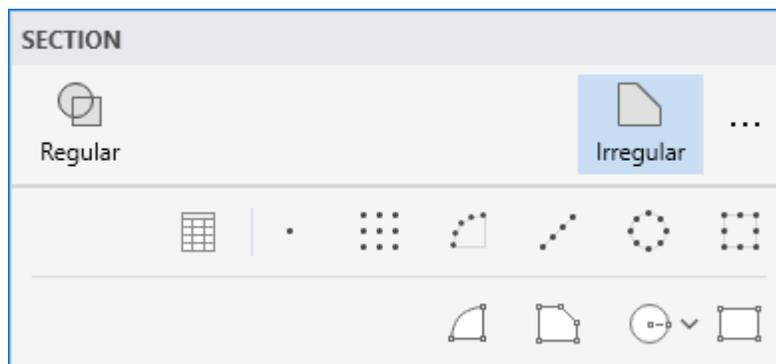
IRREGULAR section option enables the user to investigate irregularly shaped reinforced concrete sections subject to a combination of loadings. Irregular sections may contain multi-solids and multi-openings with reinforcement bars.
