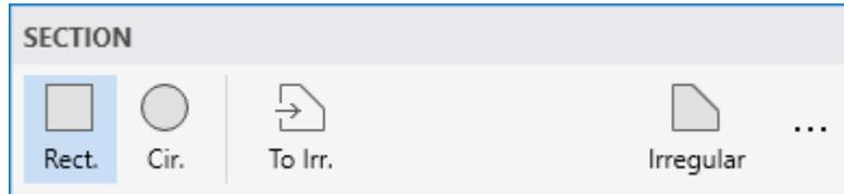
In DESIGN MODE, you can create a REGULAR section using the options available in the **Left Panel**. You can simply select the SECTION, RECTANGULAR or CIRCULAR, and enter the SIZE, BAR ARRANGEMENT, REINFORCEMENT and COVER TYPE data in the **Left Panel**. The section will automatically change according to the data entered.
