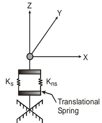
Figure 2-5 Soil Element
