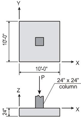
The origin of the XY plane will be located at the lower left-hand corner of the footing. Two-foot square elements will be used; thus, the grid system consists of six grid lines (i.e. five elements), two feet apart, in each direction. The concentrated load will be applied as four nodal loads (125 kip each). The finite element mesh is shown at the end of this example.
