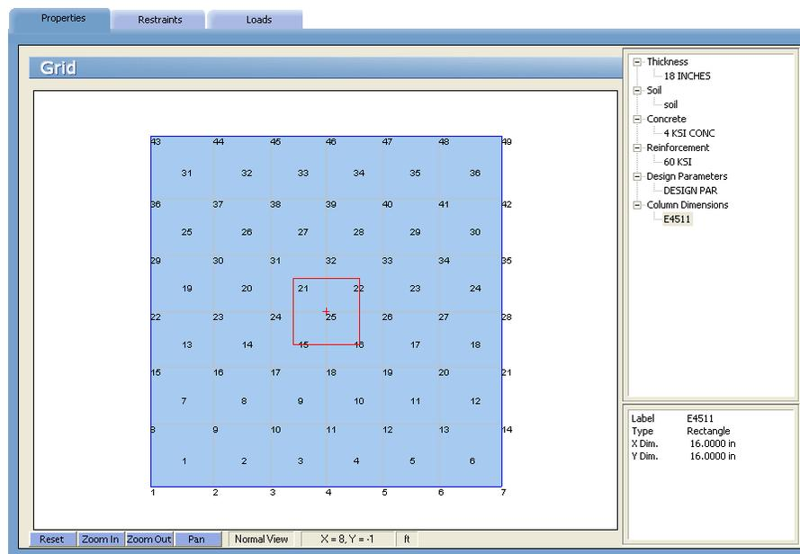
To facilitate assignment of columns, options to show the element and node labels are provided in the pop-up menu accessible by right-clicking on any blank portion of the screen.
