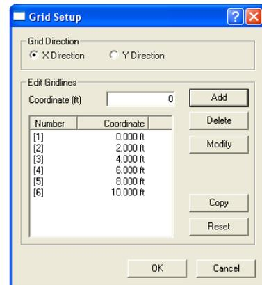
Note: New elements may be generated automatically as new grid lines are added. spMats checks the number of elements and a warning message will alert the user if the maximum allowable number of elements is exceeded. In order to solve the model, however, user needs to delete some grid lines or elements later to ensure that the number of elements is below the limit.
