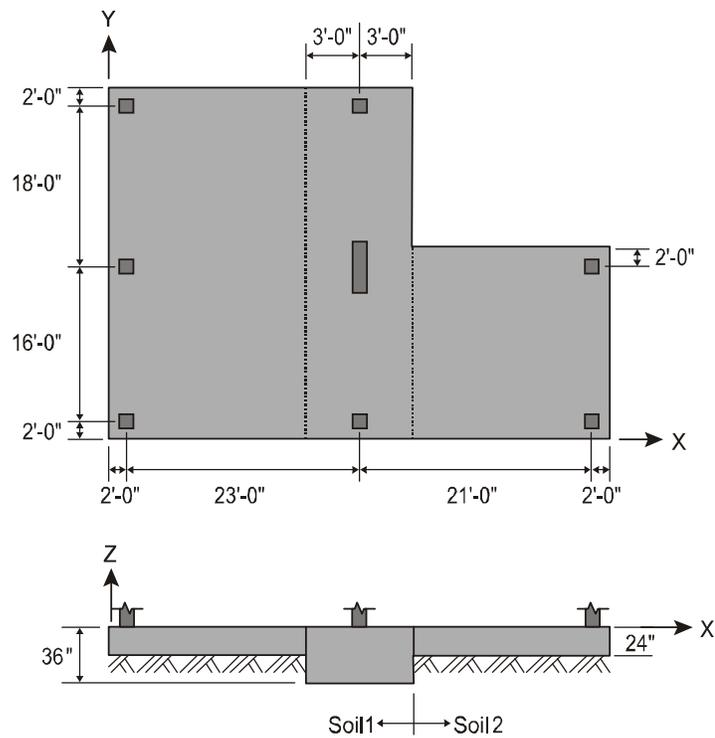
The mat is supported on two types of soil, soil-1 and soil-2, as shown in the figure. Use the following data:
