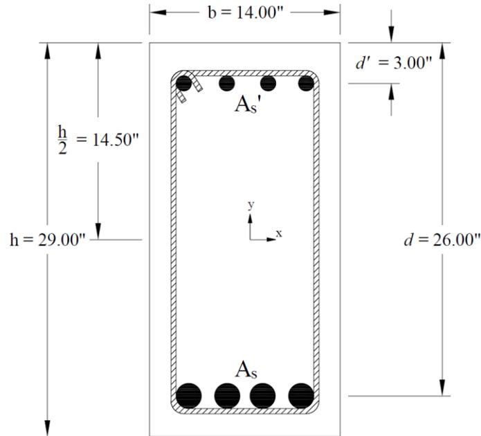
Figure 1 – Doubly Reinforced Concrete Beam Cross-Section
