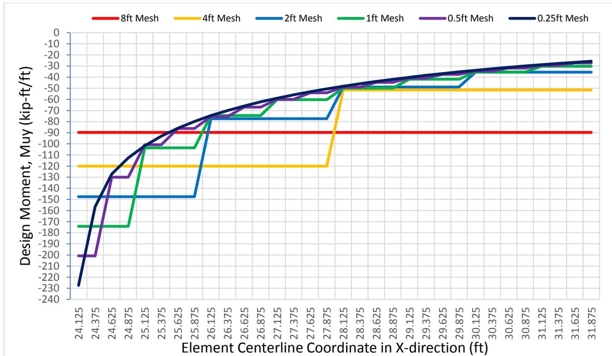
Figure 3 - Design Bottom Moment,  $M_{uy}$  (ft-kip) @  $Y=24'-0"$  between  $X=24'-0"$  and  $X=32'-0"$
