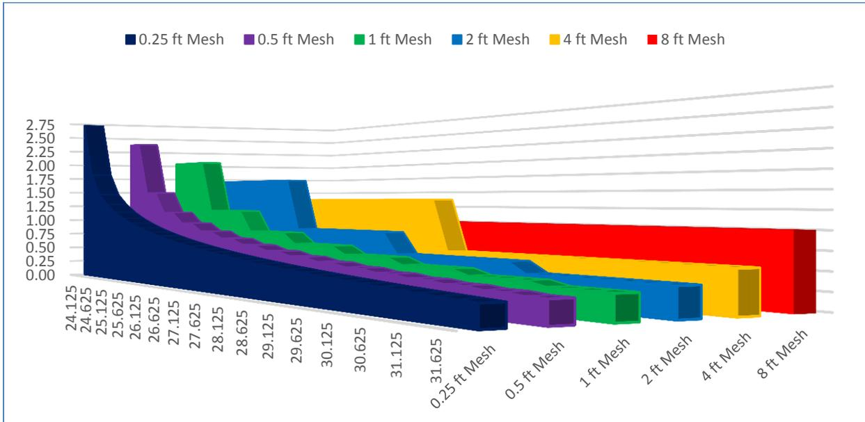
Figure 4 - Bottom Reinforcement Along Y-direction , A<sub>sy</sub> (in<sup>2</sup>) @ Y=24'-0" between X=24'-0" and X=32'-0".
