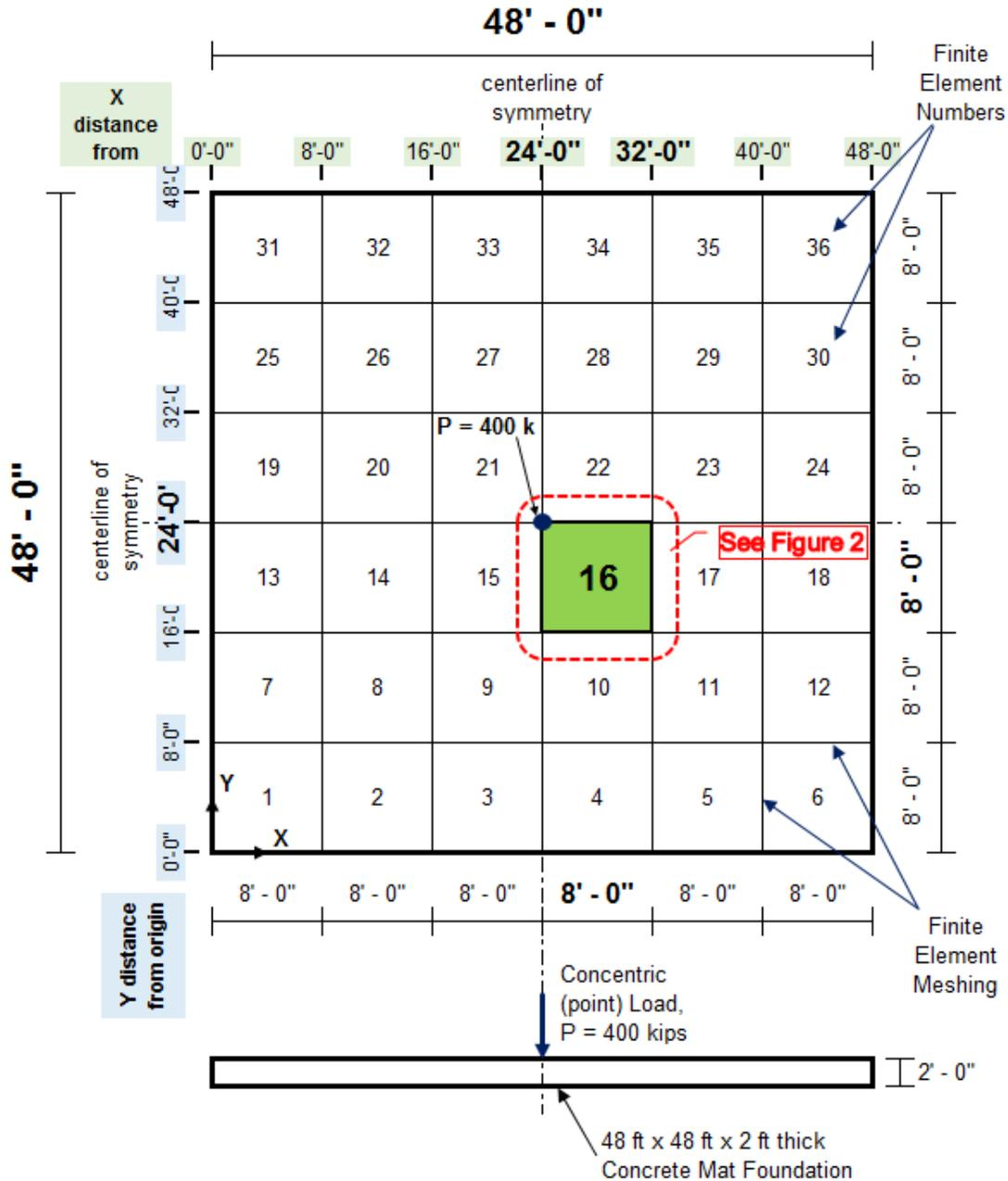
Figure 1 – Plan and Elevation View of the 48'-0" x 48'-0" x 2' deep Mat Foundation with 8 ft Finite Element Mesh
