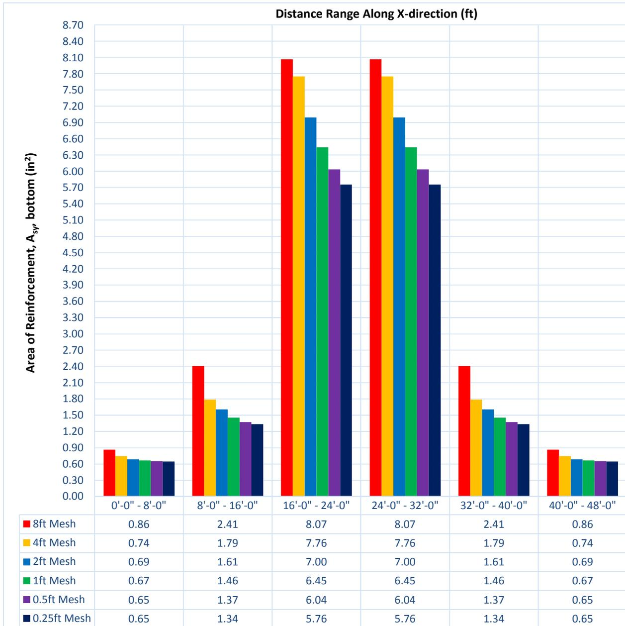
Figure 4 - Bottom Reinforcement Along Y-direction ,  $A_{sy}$  (in<sup>2</sup>) @ Y=24'-0" between X=24'-0" and X=32'-0".
