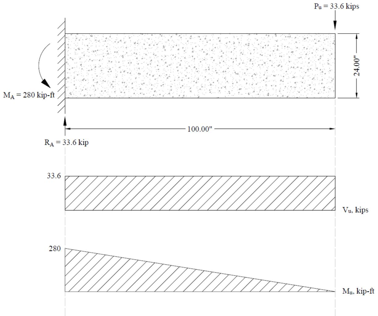
Figure 2 – Shear and Bending Moment Diagrams
