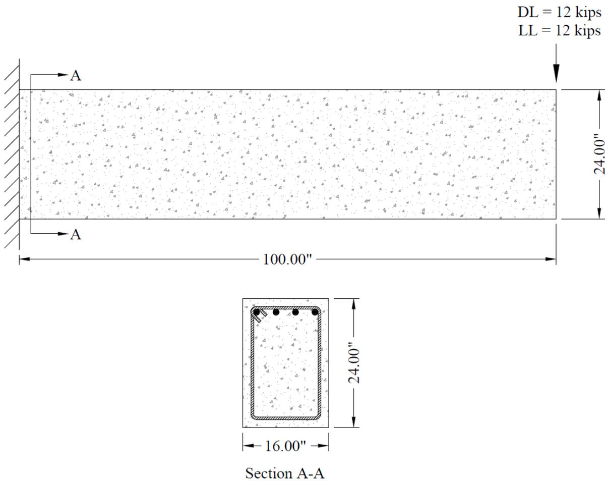
**Figure 1 – Rectangular Reinforced Concrete Cantilever Beam**
