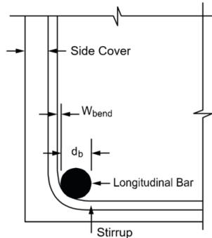
Figure 4 – Width Due to Stirrup Bend (spBeam Manual – Figure 2.21)
