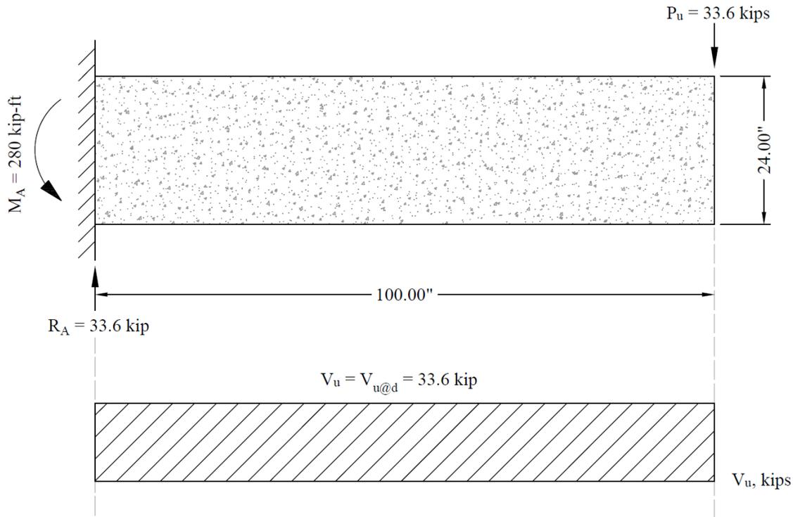
Figure 5 – Shear Diagram for Cantilever Beam
