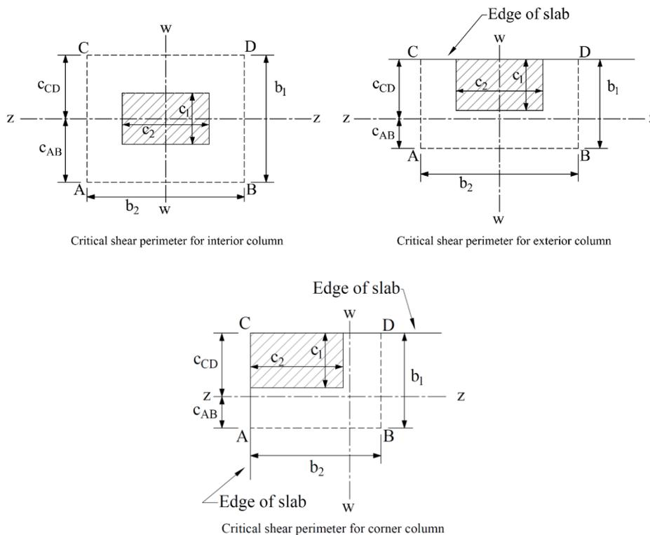
**Figure 7 – Critical Shear Perimeters for Columns**
