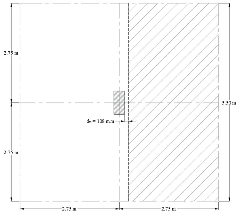
Figure 5 – Critical Section for One-Way Shear (Slab without Opening)
