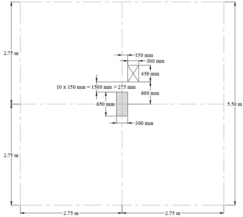
Figure 2 – Floor Opening Dimensions and Location
