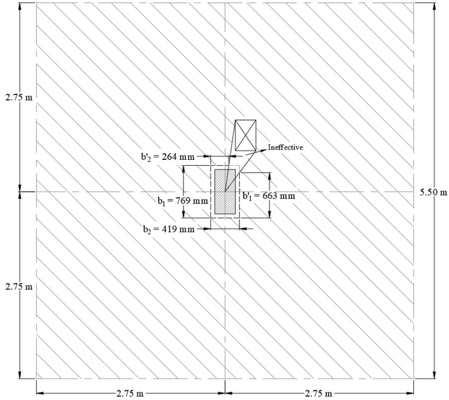
Figure 9 – Critical Section for Two-Way Shear (Slab with Opening)
