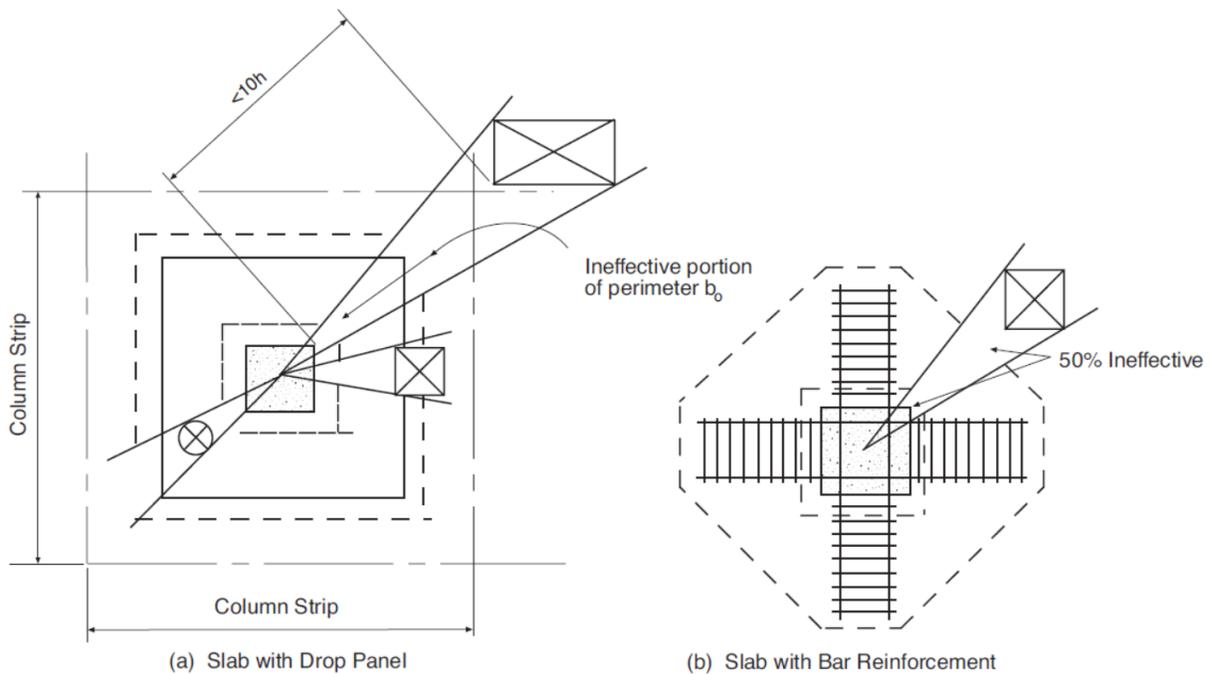
Figure 3 – Effect of Openings on Slabs Shear Strength (PCA Notes on ACI 318-11)
