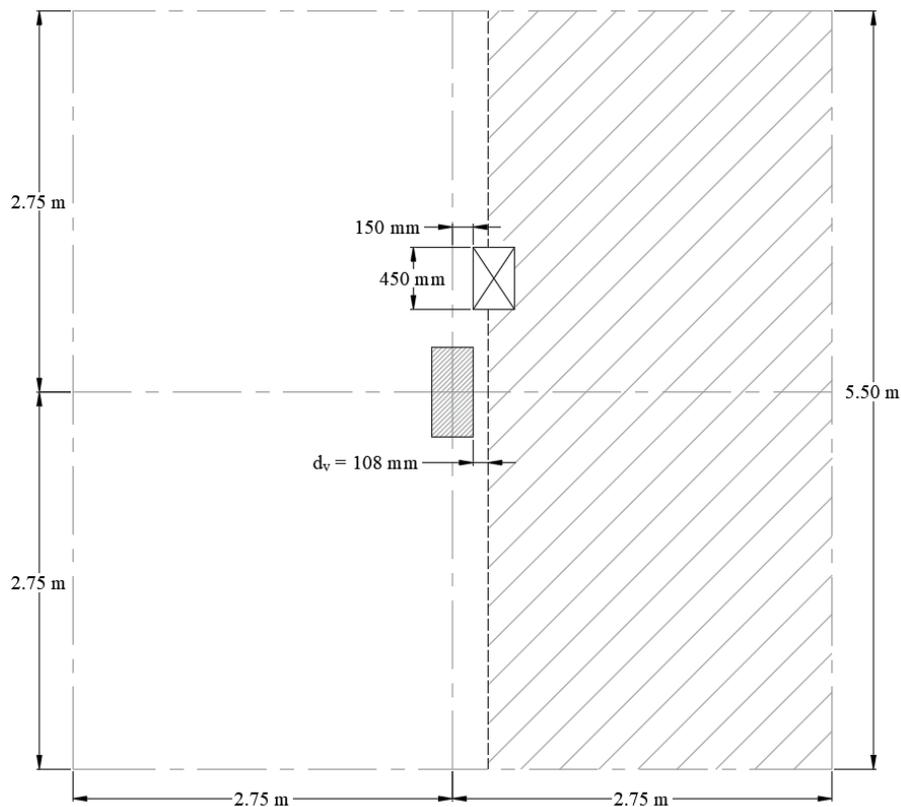
Figure 6 – Critical Section for One-Way Shear (Slab with Opening)
