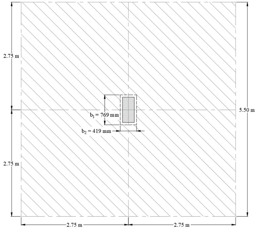
Figure 8 – Critical Section for Two-Way Punching Shear (Slab without Opening)
