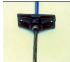
Figure 1: Tendon showing anchor, strand, and sheathing
