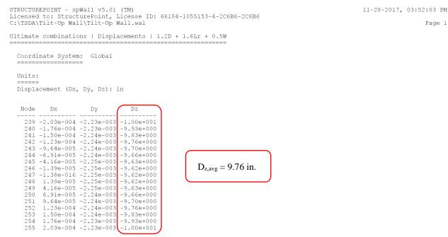
Figure 10 - Tilt-Up Wall Panel Displacement at Critical Section (Ultimate Combinations) (spWall)
