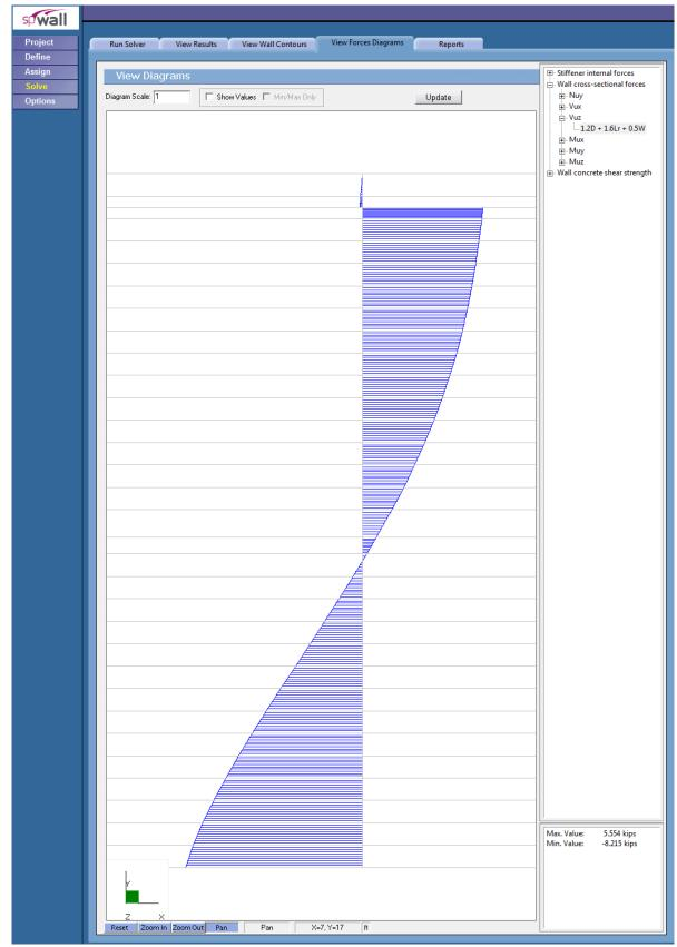
Figure 6 – Out-of-plane Shear Diagram (spWall)
