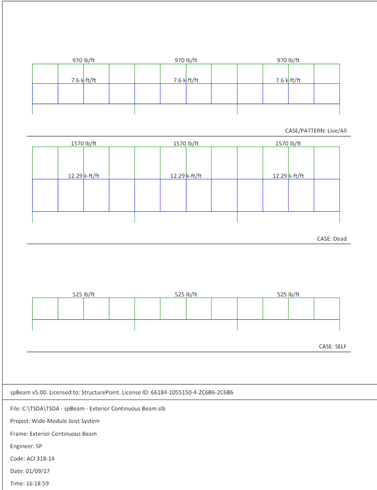
Figure 2.4.6.2 – spBeam Model – Loads (Including Live Load Patterning)
