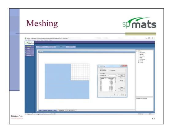
spMats breaks the system up into unique elements and nodes by utilizing a meshing or grid system. The grid can be defined gridline to gridline, or generated by specifying a starting location, the number of grids, and the spacing between each. Once the grid is generated the user can still define new gridlines at nonstandard spacing.
