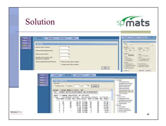
Before solving the system there are six important inputs required of the user. The maximum number of iterations along with the maximum displacement limit are the controlling factors for most typical models. The computation of reinforcement is based on either the maximum moment or the average moment within the element. This flexibility allows the engineer the ability to use industry standards.
