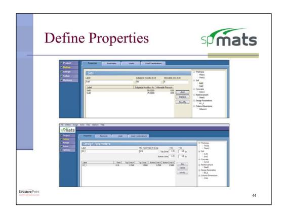
With the elements created, the system requires certain definitions to be assigned to each element. These required definitions are concrete thickness, soil properties, concrete properties, reinforcing properties, and the design parameters concrete cover and minimum reinforcing ratio.
