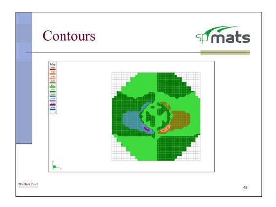
The reason that spMats is such an essential tool for mat design is that it takes the user's specifications and provides contour maps of the moments, displacements, and reinforcing required of the foundation. These contour maps give the engineer instant recognition of how the foundation will behave and the corresponding required reinforcing.
