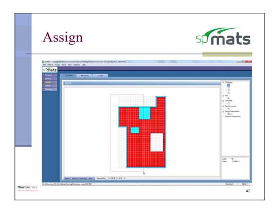
Each element is a unique part of the system that can be given any of the previously defined system definitions. When assigning these definitions, the teal elements represent a part of the meshing that has been assigned a thickness, but not the currently selected definition, red represents that the current definition is assigned, and white indicates unoccupied space. This is to allow for quick visual checks of the system.
