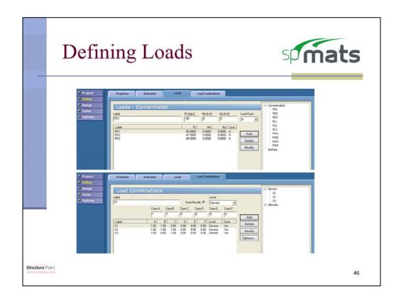
Loads acting on the mat can be modeled as either concentrated point loads or surface loads. These loads can act as a vertical force or as moments acting along the x and y directions. Each of these loads must be assigned to a load case.
