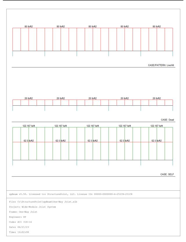
Figure 17 - spBeam Model - Loads (Including Live Load Patterning)
