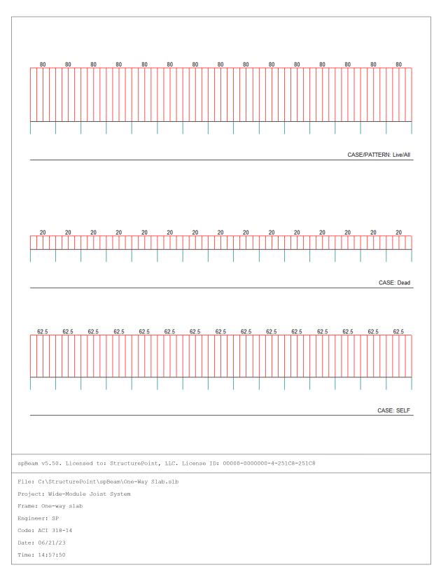
Figure 6 - spBeam Model - Loads (Including Live Load Patterning) units in lb/ft<sup>2</sup>
