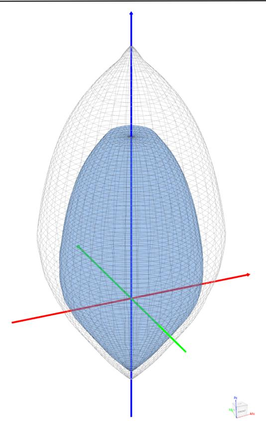
Figure 17 – Nominal & Design Interaction Diagram in Two Directions (Biaxial) (spColumn)
