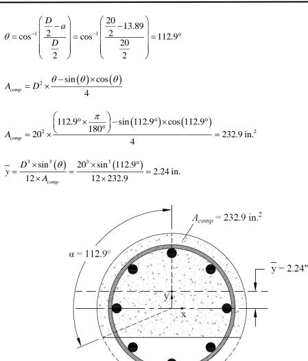
Figure 4 – Cracked Column Section Properties ( $\varepsilon_t = f_s = 0$ )
