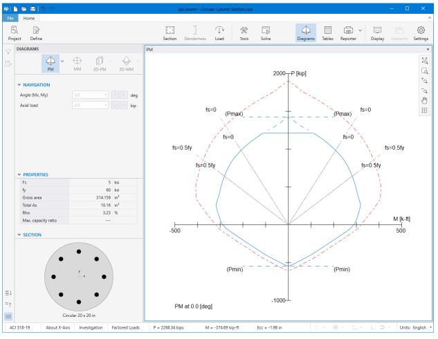
Figure 16 - Column P-M Interaction Diagram about the X-Axis (spColumn)
