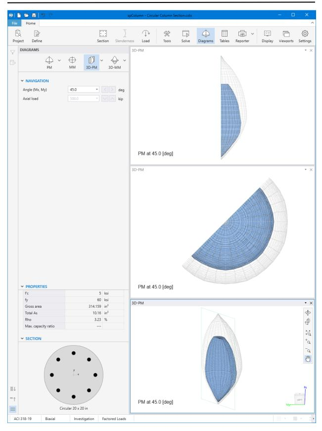
Figure 20 - Circular Column 3D Failure Surface with a Vertical Plane Cut at 45° (spColumn)
