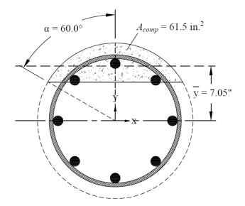
Figure 12 - Cracked Column Section Properties (Pure Moment)
