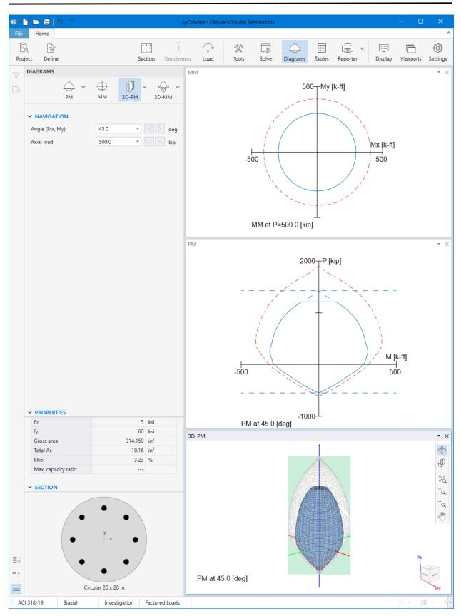
Figure 18 - Circular Column Interaction Diagram and 3D failure Surface Viewer (spColumn)
