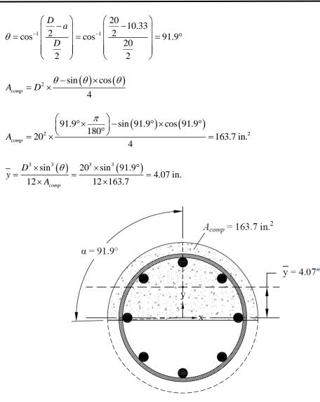
Figure 6 – Cracked Column Section Properties ( $f_s = 0.5 f_y$ )
