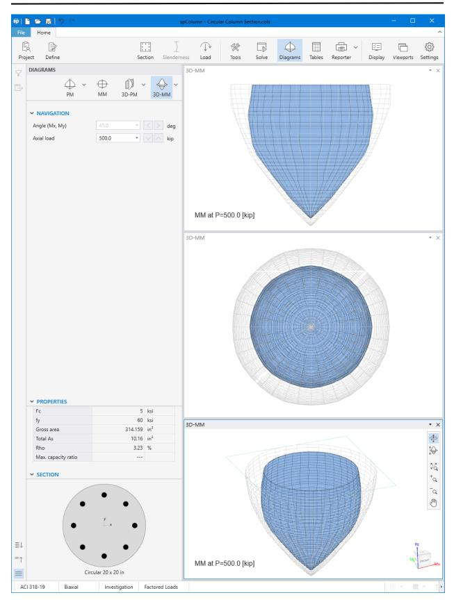
Figure 19 – Circular Column 3D Failure Surface with a Horizontal Plane Cut at P = 500 kip (spColumn)
