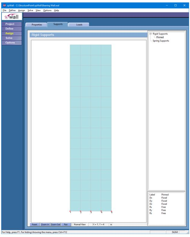
Figure 3 - Assigning Boundary Conditions for Reinforced Concrete Bearing Wall (spWall)
