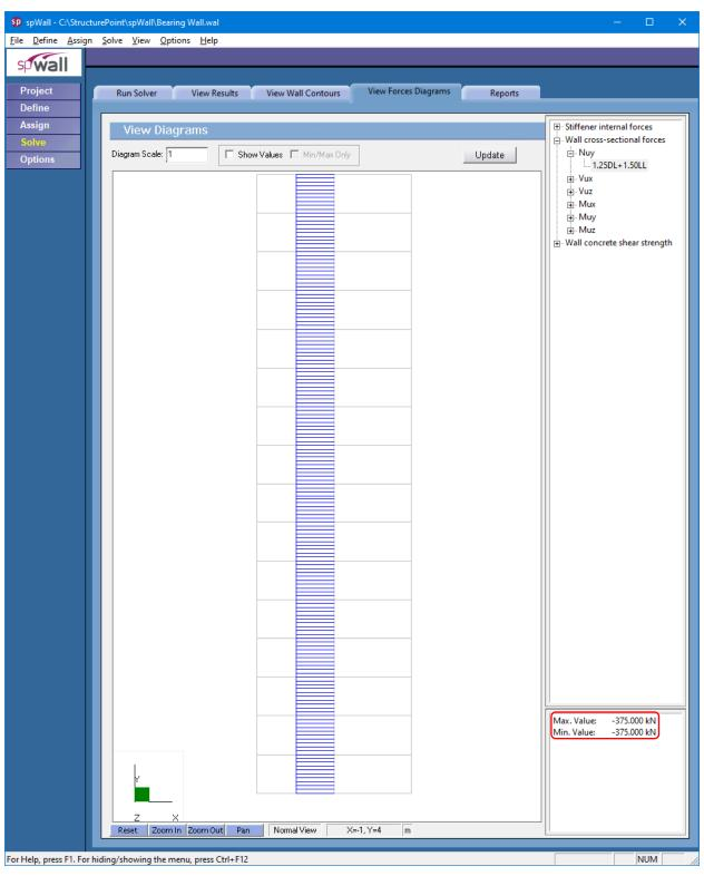
Figure 6 - Reinforced Concrete Bearing Wall Axial Load Diagram (spWall)
