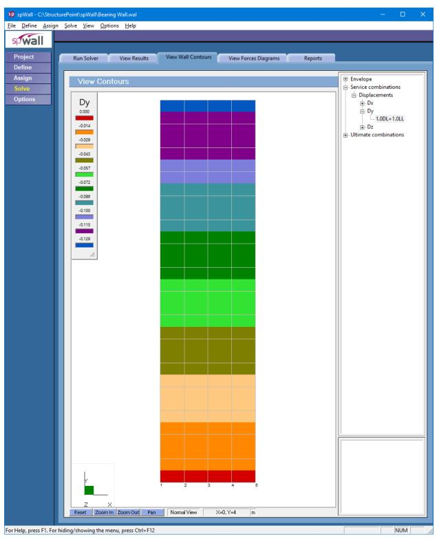
Figure 5 - Reinforced Concrete Bearing Wall Vertical Displacement Contour (In-Plane) (spWall)
