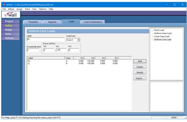
Figure 2 - Defining Loads for Reinforced Concrete Bearing Wall (spWall)
