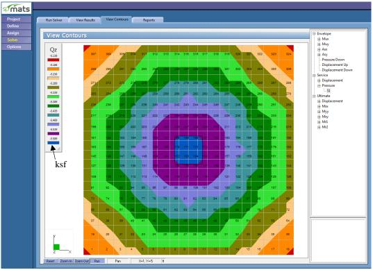
Figure 9 – Footing Soil Pressure Contour (spMats)
