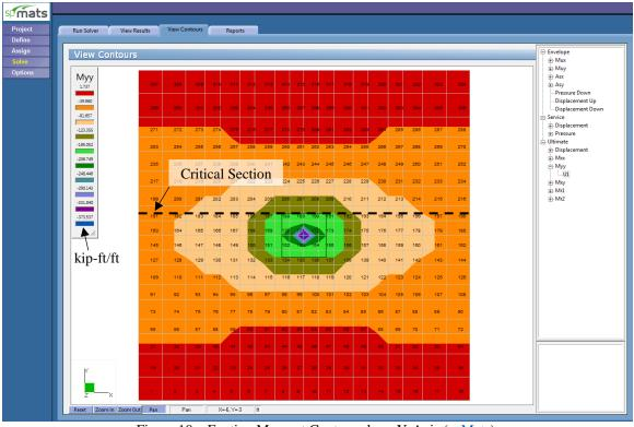
Figure 10 – Footing Moment Contour along Y-Axis (spMats)
