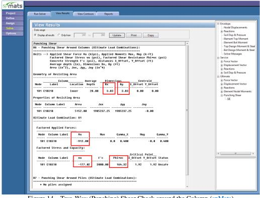
Figure 14 - Two-Way (Punching) Shear Check around the Column (spMats)
