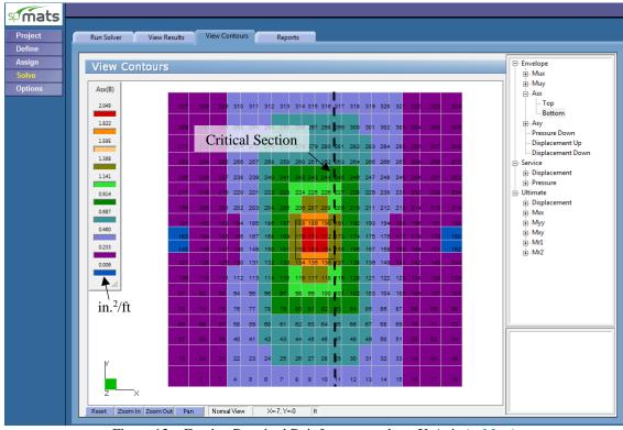
Figure 12 - Footing Required Reinforcement along X-Axis (spMats)
