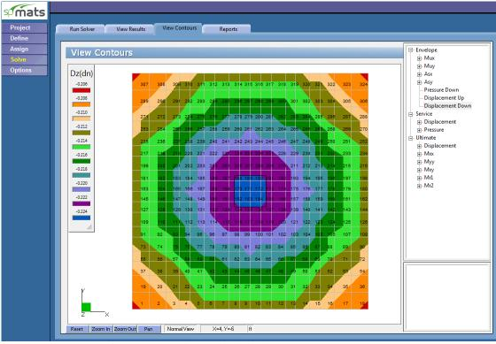
Figure 13 – Footing Vertical Displacement Contour (spMats)
