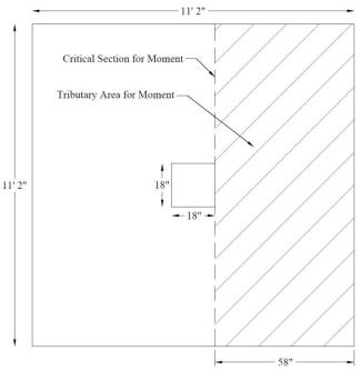
Figure 4 - Critical Section for Moment
