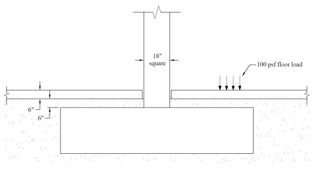
Figure 1 - Reinforced Concrete Spread Footing
