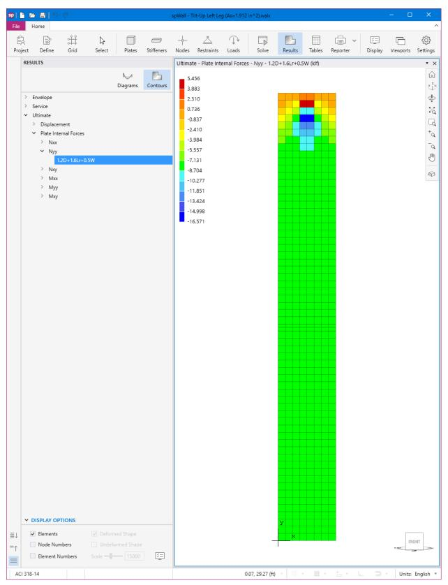
Figure 25 - Factored Axial Forces Contour Normal to the Left Design Strip Cross-Section (spWall)
