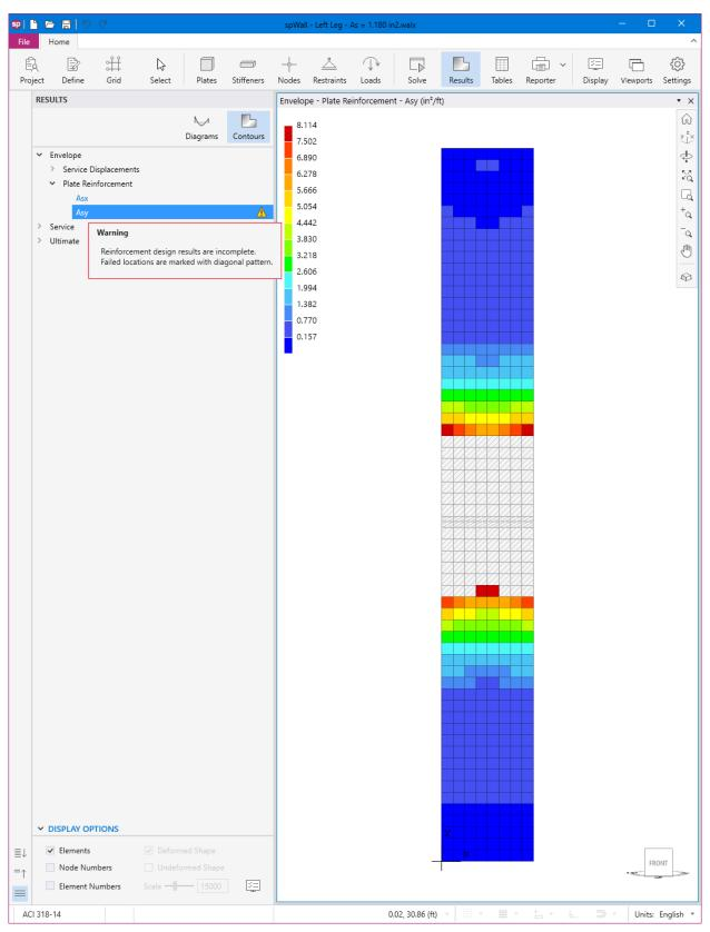
Figure 24 – Failing Reinforcement Error (spWall)
