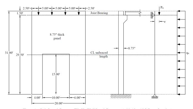
Figure 1 – Reinforced Concrete Tilt-Up Wall Panel Geometry (with 10 x 15 ft Door Opening)
