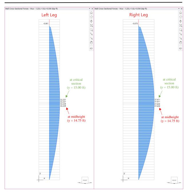
Figure 11 – Tilt-Up Wall Panel with Opening Moment Diagram (spWall)
