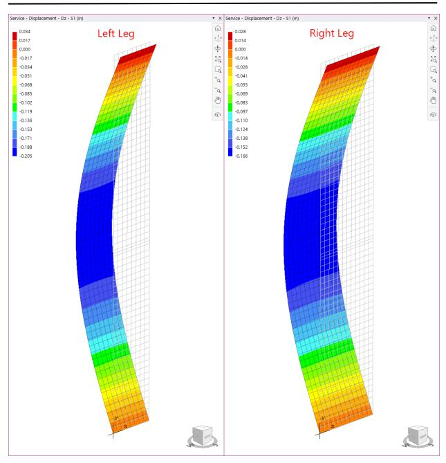
Figure 9 - Tilt-Up Wall Panel Service Lateral Displacement Contour (Out-of-Plane) (spWall)
