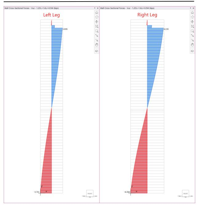
Figure 10 – Out-of-plane Shear Diagram (spWall)
