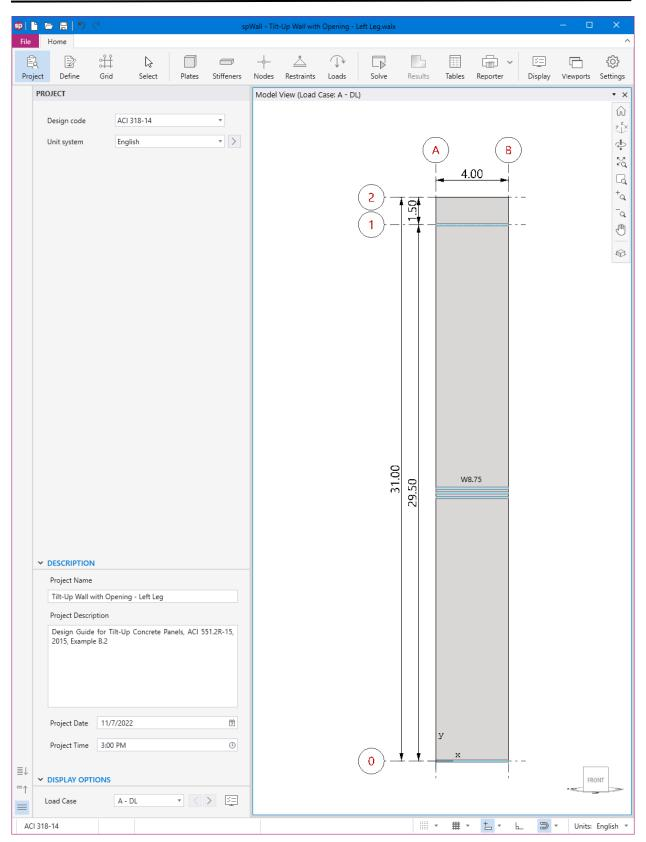
Figure 3 – spWall Interface
