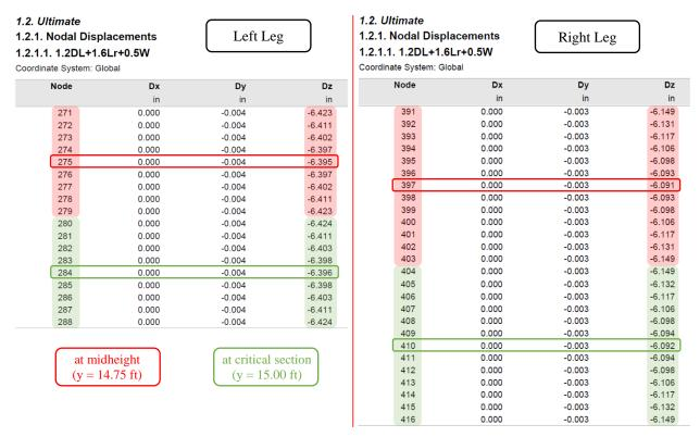
Figure 13 – Tilt-Up Wall Panel with Opening Displacement at Critical Sections (Ultimate Combinations) (spWall)
