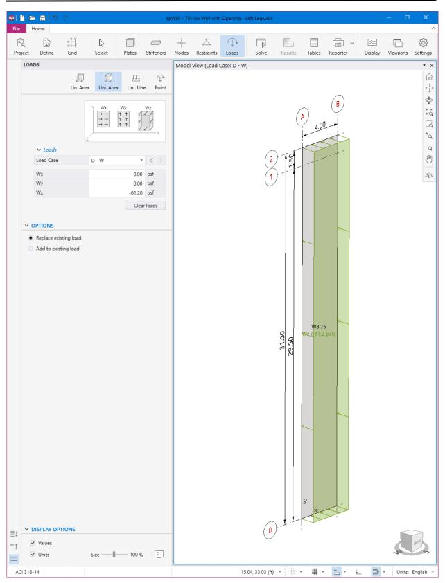
Figure 6 – Assigning Wind Loads for Tilt-Up Wall (spWall)
