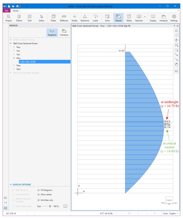
Figure 18 – Tilt-Up Wall Panel with Opening Moment Diagram – Exact Geometry and Loads (spWall)
