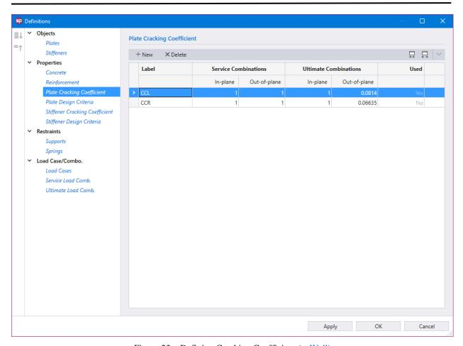
Figure 23 – Defining Cracking Coefficient (spWall)
