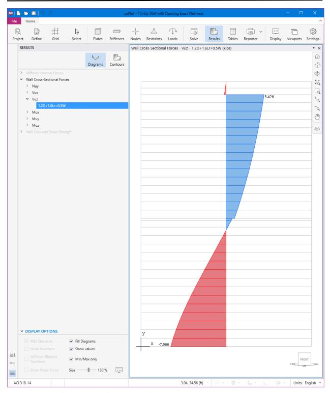
Figure 17 - Out-of-plane Shear Diagram - Exact Geometry and Loads (spWall)
