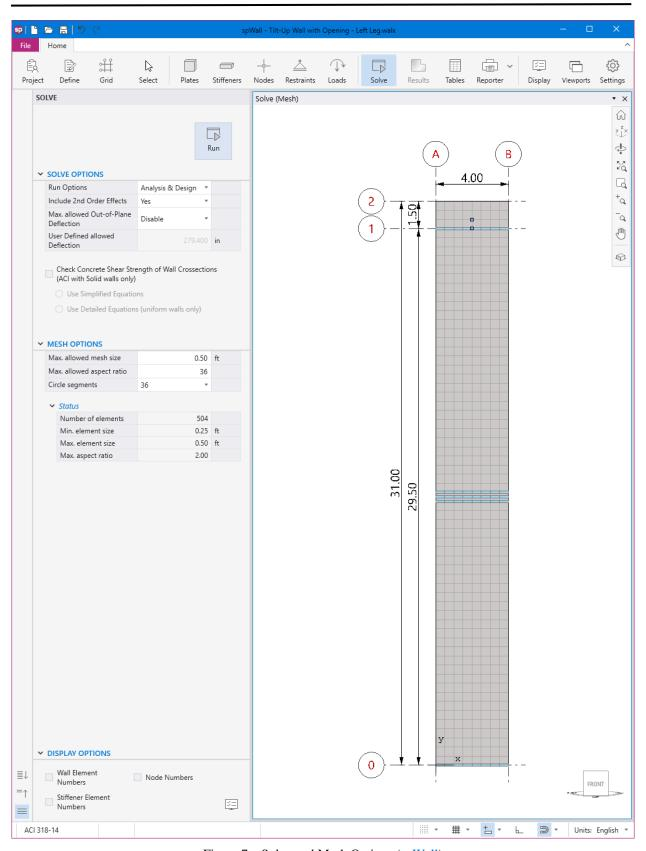
Figure 7 – Solve and Mesh Options (spWall)
