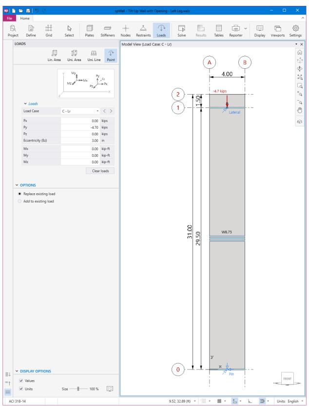
Figure 5 – Assigning Roof Live Loads for Tilt-Up Wall (spWall)
