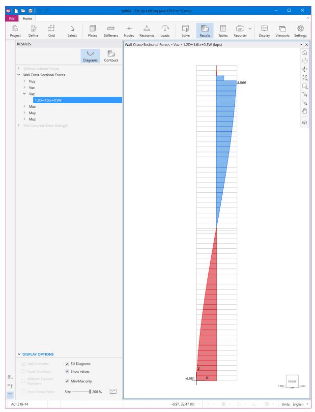
Figure 28 – Out-of-plane Shear Diagram (spWall)
