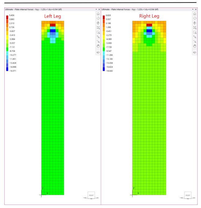
Figure 8 – Factored Axial Forces Contour Normal to Tilt-Up Wall Panel Design Strips Cross-Sections (spWall)
