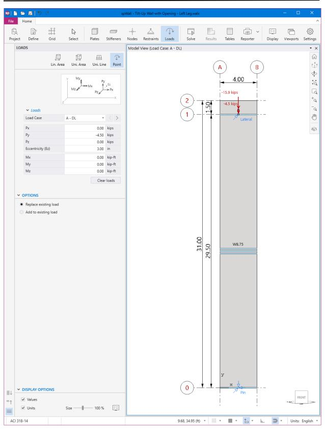
Figure 4 – Assigning Roof Dead Loads for Tilt-Up Wall (spWall)
