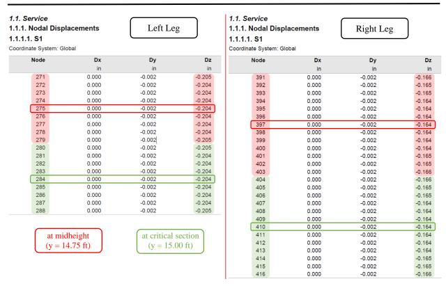
Figure 12 – Tilt-Up Wall Panel with Opening Displacement at Critical Sections (Service Combinations) (spWall)
