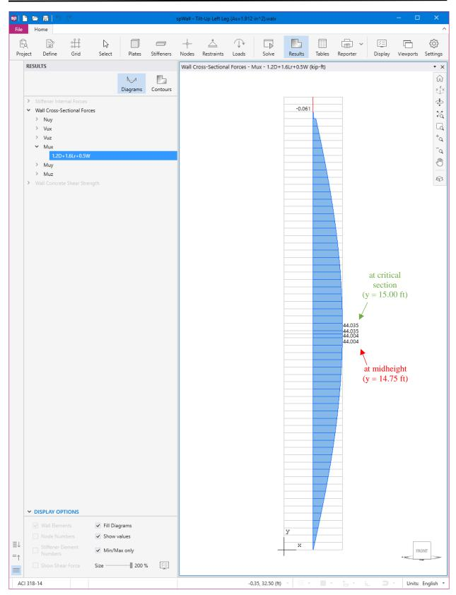
Figure 29 - Tilt-Up Wall Panel with Opening Moment Diagram (spWall)
