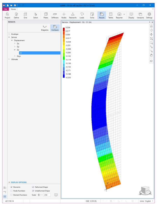
Figure 26 - Service Lateral Displacement Contour (Out-of-Plane) (spWall)
