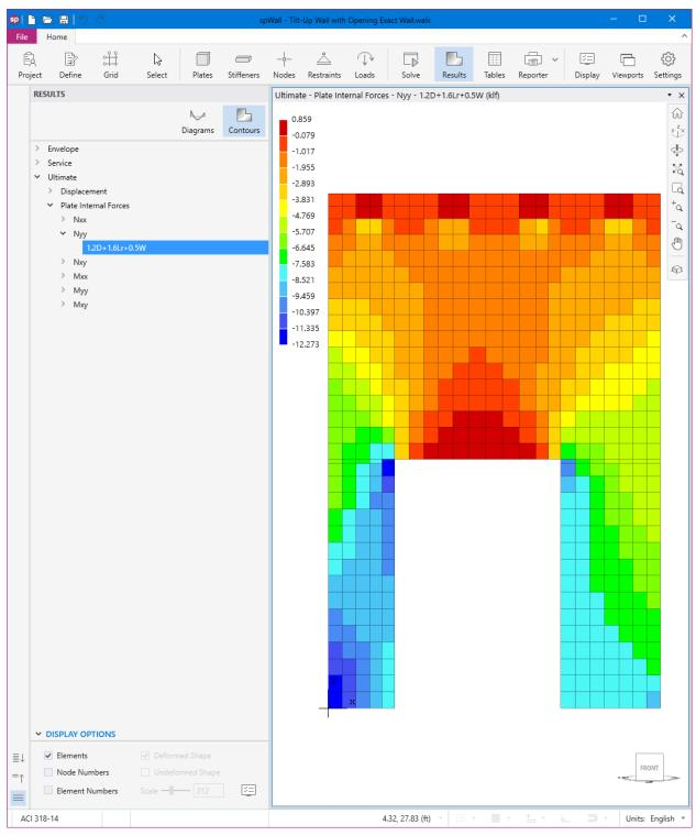
Figure 15 - Factored Axial Forces Contour - Exact Geometry and Loads (spWall)
