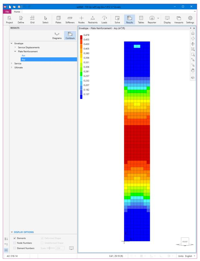
Figure 27 – Vertical Reinforcement Contour (in. 2/ft) (spWall)
