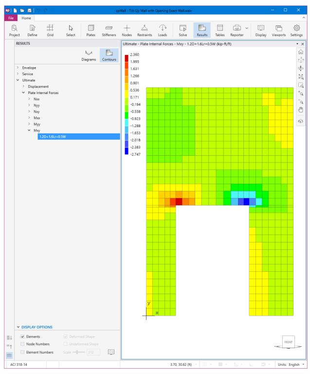
Figure 22 - Tilt-Up Wall Panel with Opening Torsional Moment Contour (spWall)
