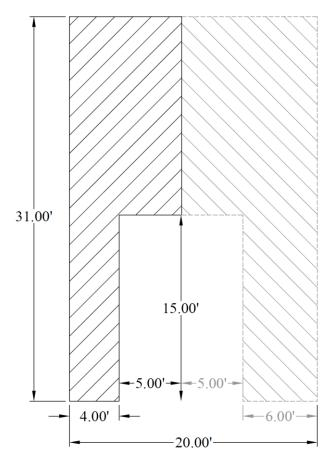
Figure 2 – Tilt-Up Design Strips Tributary Widths for Loads
