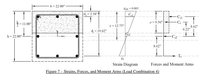
The following procedure is used to determine the nominal moment capacity by setting the design axial load capacity,  $\phi P_n$ , equal to the applied axial load,  $P_u$  and iterating on the location of the neutral axis.
