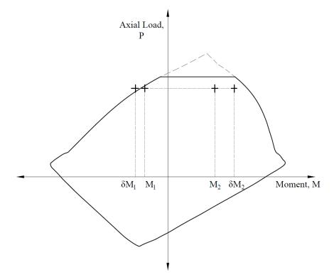
Figure 6 – Column Interaction Diagram for Unsymmetrical Section
