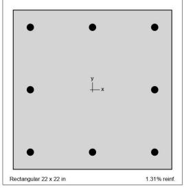
Figure 1: Column section
