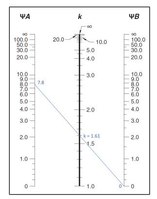
Figure 4 – Effective Length Factor (k) Calculations for Interior Columns
