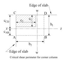
Figure 18 - Critical Shear Perimeters for Columns
