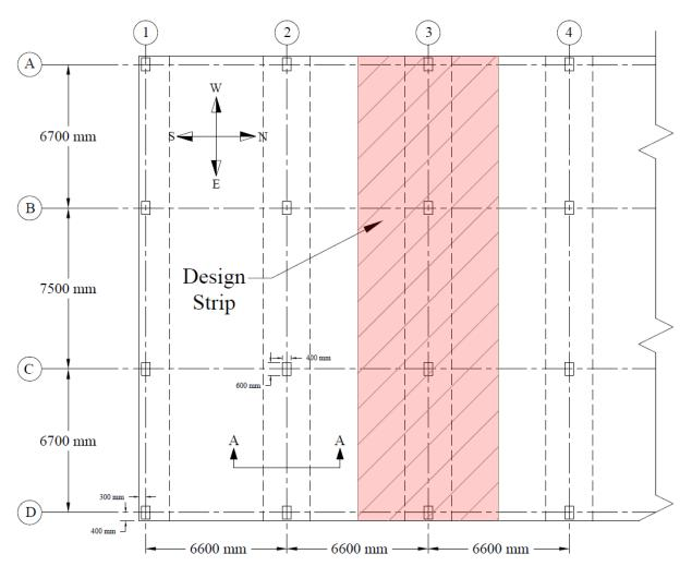
Figure 5 – Two-Way Slab with Slab Bands
