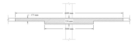
Figure 14 – Slab-Beam in the Direction of Analysis
