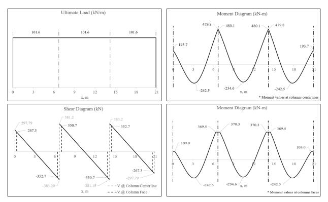
Figure 17 - Positive and Negative Design Moments for Slab-Beam (All Spans Loaded with Full Factored Live Load)
