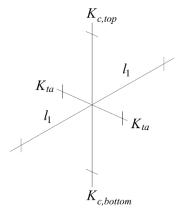
Figure 15 - Equivalent Column Stiffness
