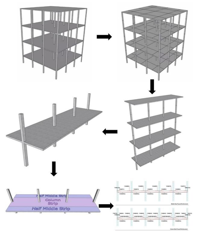
Figure 11 – Elastic (Equivalent) Frame Methodology
