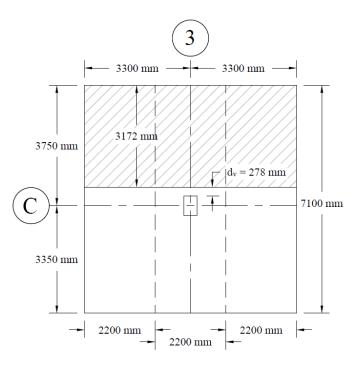
Figure 6 - Critical Sections for One-Way Shear
