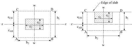
Critical shear perimeter for interior column
