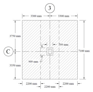
Figure 7 – Critical Section for Two-Way Shear
