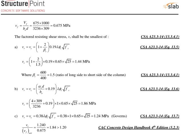
Slab band thickness of 350 mm is adequate for two-way shear for the critical section (from the edge of the column).
